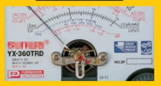
The meter part is the most important for the Analog Multitester. To prevent drop shock damage to the meter, the genuine Japanese Sanwa YX360TRF features a function called DROP PROOF. DROP PROOF only supports a taut-band type meter.
